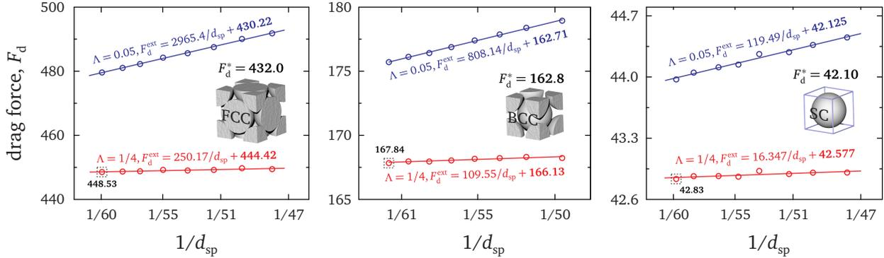
FIG. 5. Examples of extrapolation of drag values towards the infinitely-high discretization resolution assuming the solution convergence rate of  $-1$ . The shown results are for the FCC, BCC, and SC packings of touching spheres. All extrapolation results in this study are obtained with  $\Lambda = 0.05$ .
