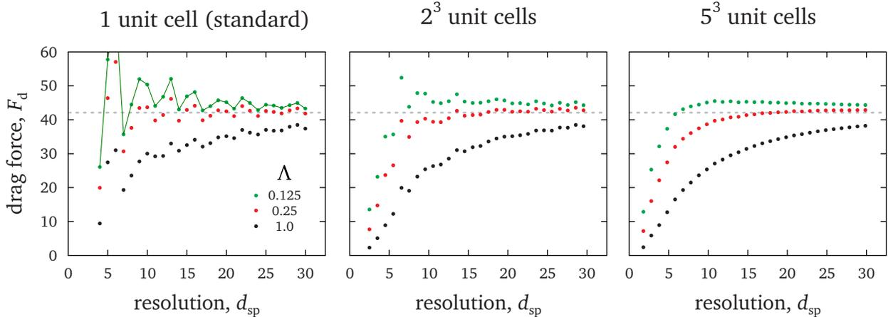
FIG. 1. Drag force vs. discretization resolution (in lattice units per sphere diameter) for simple cubic packing of touching spheres with  $\varepsilon \approx 0.476$ . Green, red, and black colors denote  $\Lambda = 0.125$ , 0.25, and 1.0, respectively. Reference drag value for this geometry is 42.1 (dashed line).
