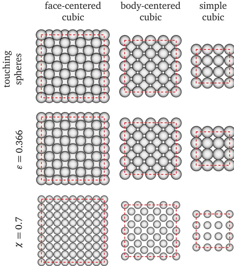
FIG. 2. Three packing types used in the simulations with unit cells replicated 4 times along each direction; the actual simulation domain is indicated with the red dashed lines. The middle row shows packings of fixed porosity ( $\varepsilon = 0.366$ ) while the top and bottom rows depict touching and diluted packings, respectively.
