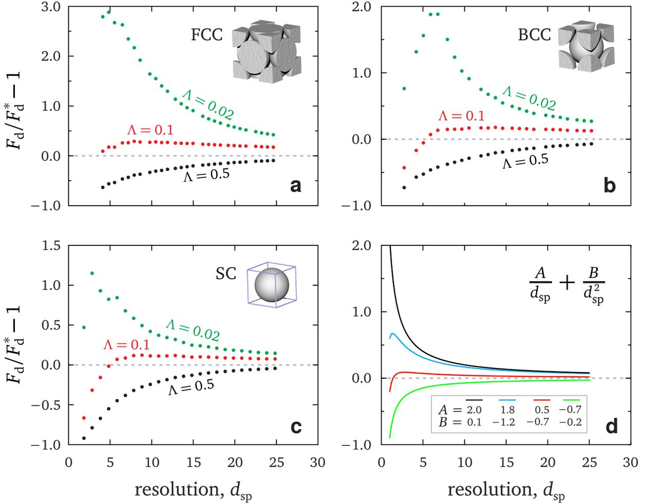
FIG. 3. a–c: Relative drag force error as a function of discretization resolution for FCC, BCC, SC packings of touching spheres; the dependencies are shown for three  $\Lambda$  values. d: a simple model that mimics variation of the quadratic and linear error convergence rates with resolution; shown are four different combinations of model parameters  $A$  and  $B$ .
